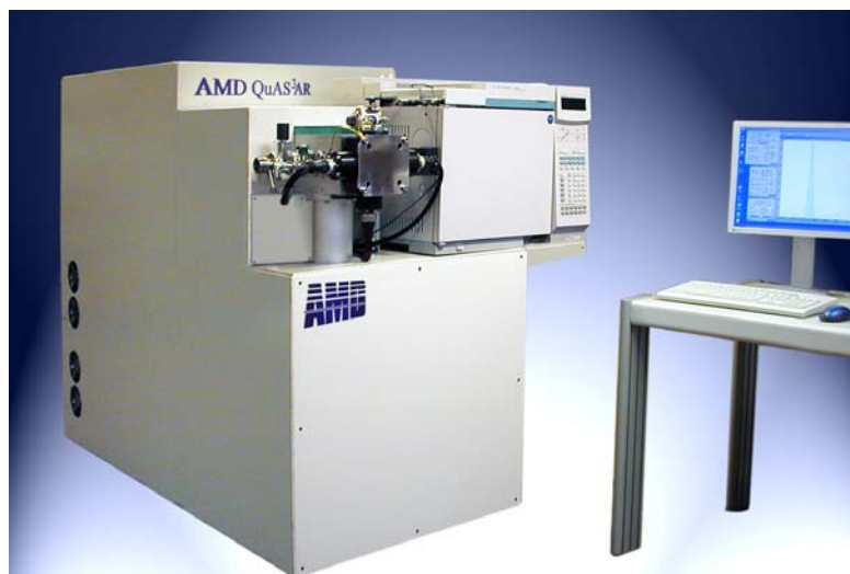
GC/MS Configuration with EI ion source and DIP/DEI sample introduction
