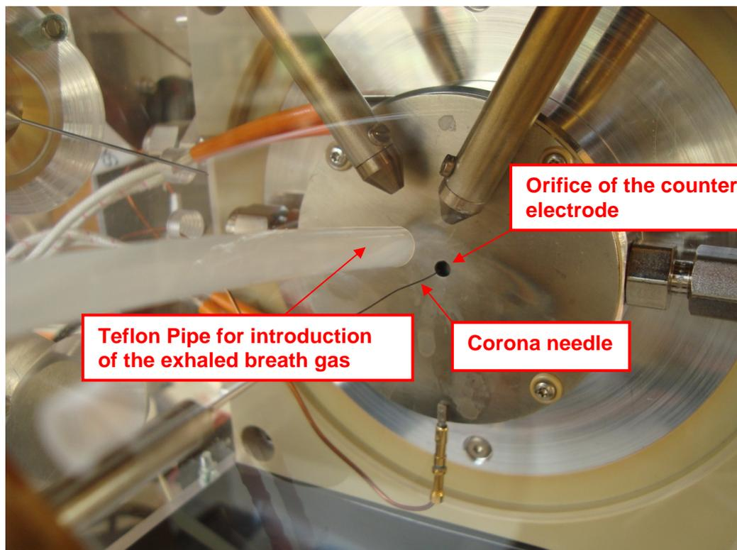
**Fig. 1 In-side view of the API chamber**
