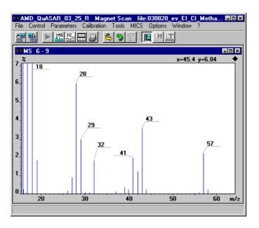
A **superimposed EI – CI** mass spectrum has been produced in preparation for an analytical GC/MS run.
