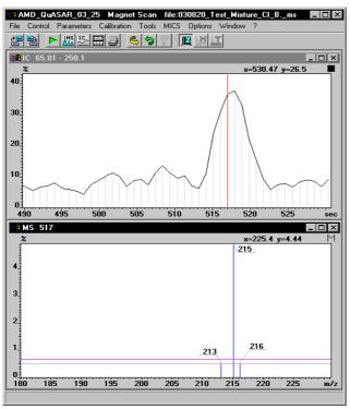
The gas chromatogram represents the same test mixture for optimization of the GC/MS conditions as above but produced here in EI only mode. Again, the last peak in the chromatogram represents the compound dodecane acid methylester.
