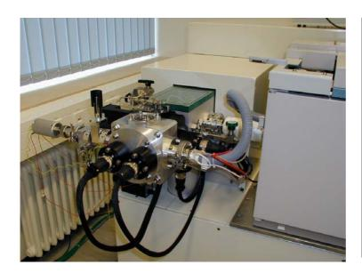
Simultaneous or alternating recording of ions from independent CI and standard EI ion source in GC/MS mode allows to combine the information content of EI spectra and CI spectra in one GC/MS run. This unique and new methodology enhances the effectiveness of GC/MS significantly.
