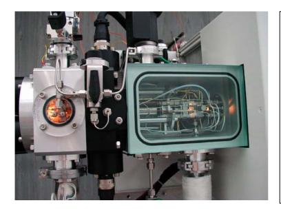
**Top view** on **independent EI** and **CI** ion sources in **simultaneous** operation
