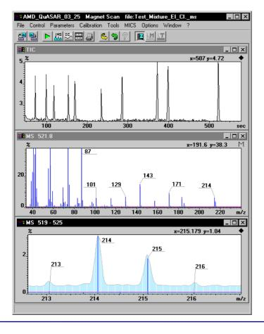
**Superimposed EI – CI** mass spectra have been produced in **GC/MS mode** by **simultaneous recording** of ions arising from independent CI and standard EI ion source
