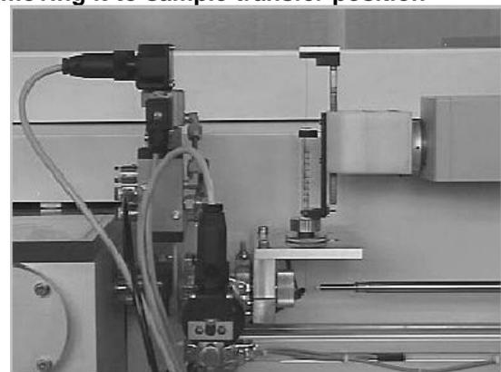
Figure 7: Sample transfer from syringe to DCI-wire
